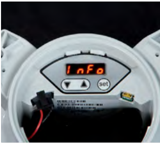
ON-BOARD USER INTERFACE Replaceable and recyclable NiMH batteries with extreme temperature range and 5-year life expectancy.
